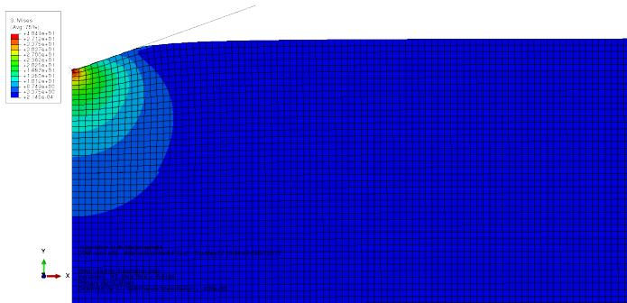
Figure 1.34: Screenshot (with a zoom in on the contact area) of the Von Mises stress distribution at maximum load.
