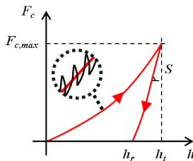
Figure 1.16: Schematic of the dynamic loading cycle.
