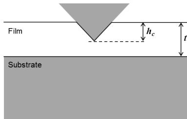
Figure 1.23: *Indentation penetration of a thin film on a sample.*
