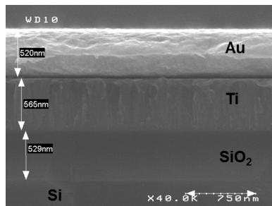
Figure 1.20: SEM cross-sectional observation of a multilayer sample.
