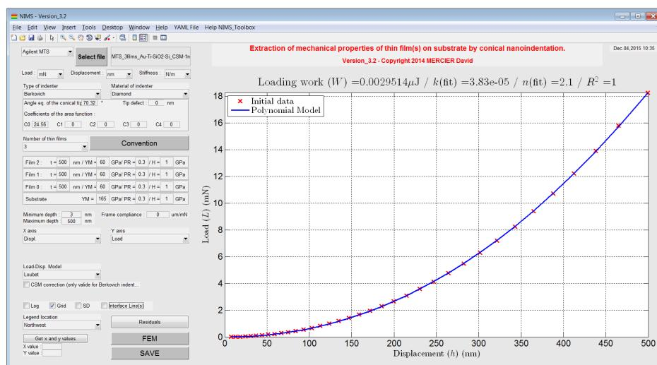
Figure 1.3: Plot of the load-displacement curve after loading of data.
