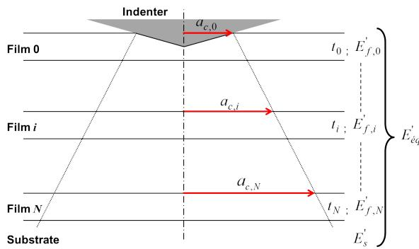
Figure 1.25: Schematic of elastic multilayer model.
