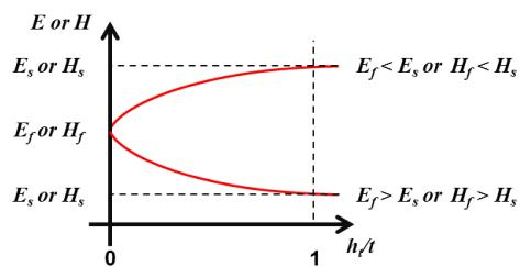
Figure 1.21: Typical evolution of Young's modulus and hardness for a coated specimen in function of the normalized indentation depth.
