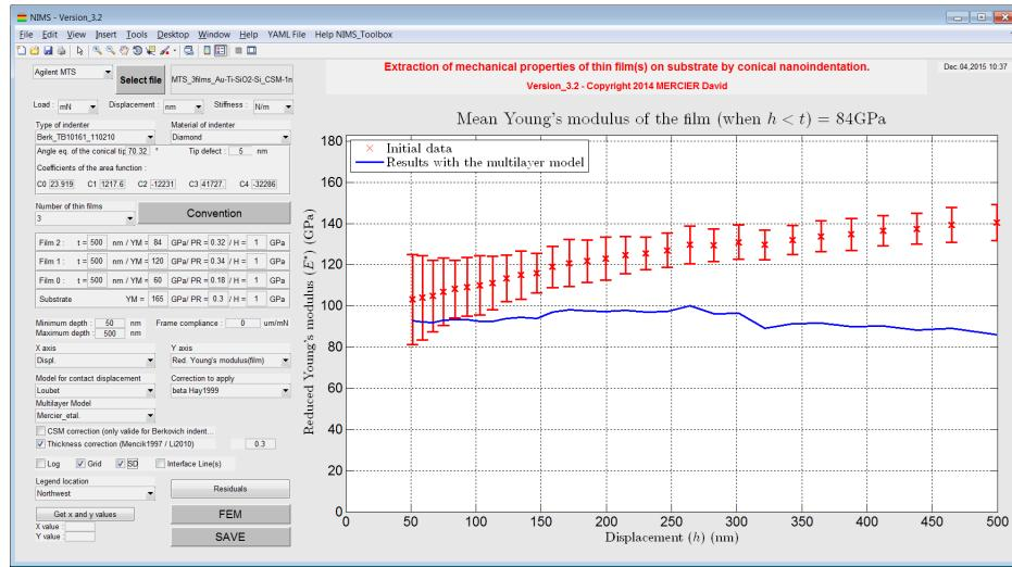
Figure 1.6: Plot of the evolution of the Young's modulus of the film with the elastic multilayer model in function of the indentation depth.
