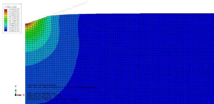
Figure 1.35: Screenshot (with a zoom in on the contact area) of the magnitude of the displacement at maximum load.
