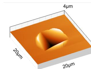
Figure 1.14: Residual topography of a Berkovitch indent in PVD Gold thin film (500nm thick) with “pile-up” surrounding the indent, measured by atomic force microscopy.
