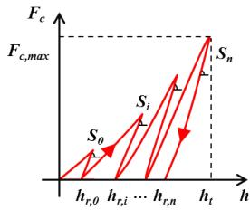
Figure 1.11: *Schematic of indentation load-displacement curve with the multiple point unload method (here  $n$  points).*
