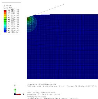
Figure 1.33: Screenshot of the Von Mises stress distribution at maximum load.
