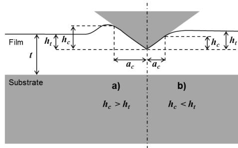
Figure 1.22: Schematic depiction of a) “pile-up” and b) “sink-in” observed during thin film indentation.
