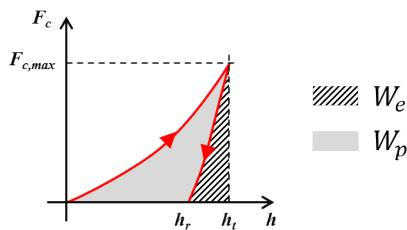
Figure 1.19: Schematic representation of indentation load–displacement curves with definition of different works of indentation.
