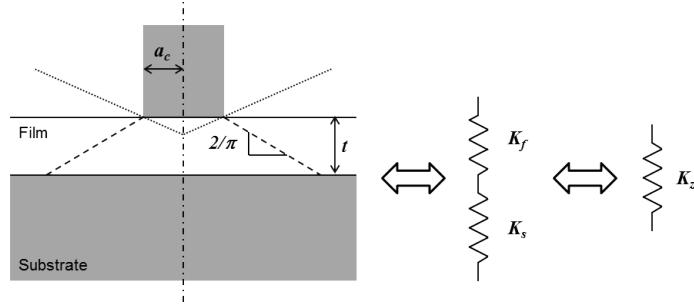
Figure 1.24: *Schematic description of the bilayer model of Bec et al.*
