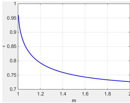
Figure 1.15: Evolution of  $\epsilon$  in function of the power law exponent  $m$  of the unloading curve.
