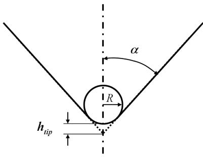
Figure 1.29: Scheme of a cono-spherical indenter.
