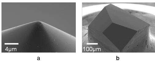
Figure 1.8: a) Conical indenter (45°) and b) Berkovich indenter.
