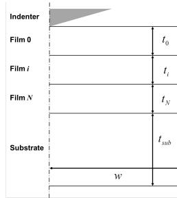
Figure 1.28: Geometry of the sample in the FEM model.
