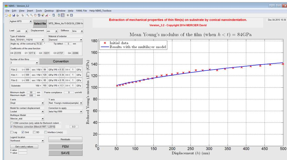
Figure 1.5: Plot of the evolution of the Young's modulus of the sample with the elastic multilayer model in function of the indentation depth.
