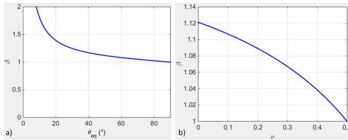
Figure 1.18: Plots of beta Hay : a) in function of the half-angle of the conical indenter (for a Poisson's ratio of 0.3), and b) in function of the Poisson's ratio for a Berkovich indenter.
