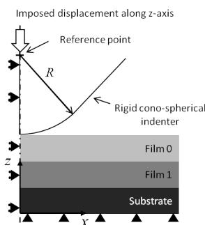
Figure 1.31: Schematic of boundaries conditions used in the FE model.
