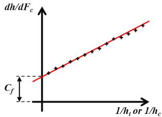
Figure 1.12: Schematic of the plot to determine the frame compliance.
