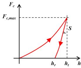
Figure 1.10: *Schematic of indentation load-displacement curve.*
