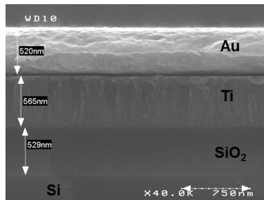
Figure 1.27: SEM cross-sectional observation of a multilayer sample.
