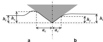
Figure 1.13: Schematic of indentation contact topography : a) “pile-up” and b) “sink-in”.
